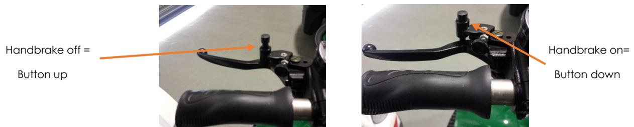
Fig. 6: Handbrake off
