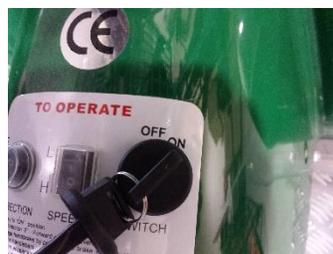
Fig. 4: Key switch (ignition)
