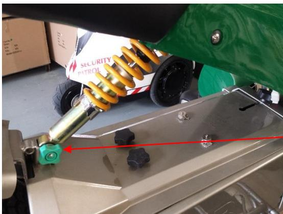
Fig. 5: Rear Shock Absorber
